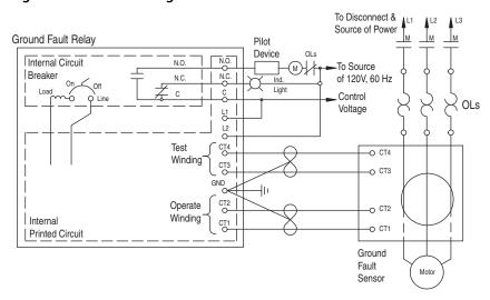
Figure 2 - Class II with High Current Inhibit Circuit (1)
